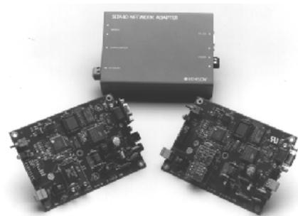
The SLTA-10 is a NSI-compatible LonTalk adapter with a RS232 interface to the host computer.
