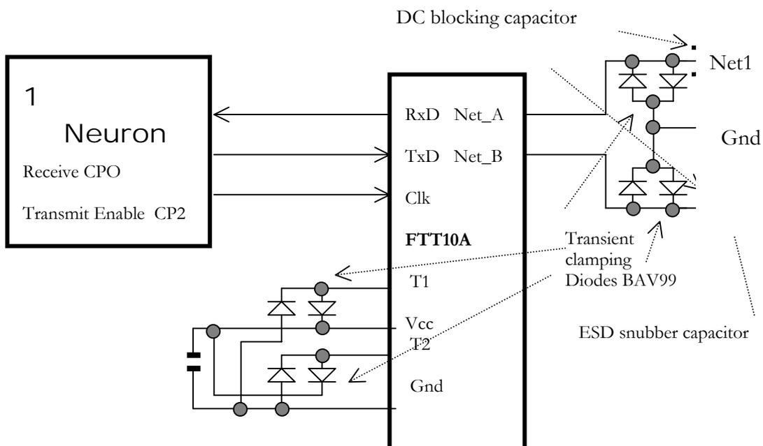
The network connection (NET1 and NET2) is polarity insensitive and therefore either of the two twisted pair wires can be connected to either of these two network connections.
