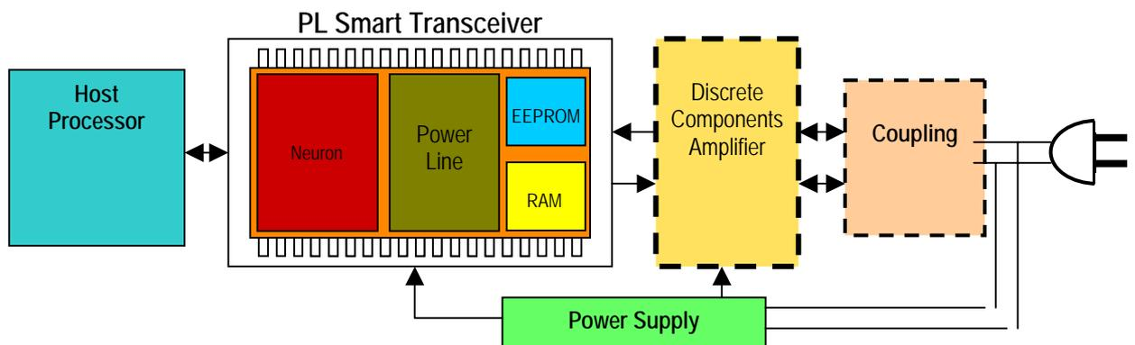
The power amplifier is an around-50 discrete components design (mostly resistors and condensators along with a small number of transistors).
