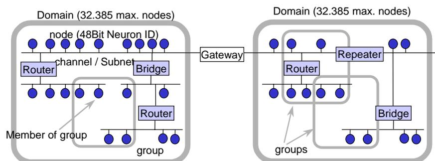
**Router:** selectively forwards packets between two channels of same or different physical media. (e.g. RS485 to FTT10A).
