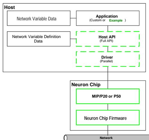
The MIP is delivered as a Neuron C library that allows the NodeBuilder software to include system calls for the MIP. The NodeBuilder is needed to create a ROM image that executes on the Neuron chip.
