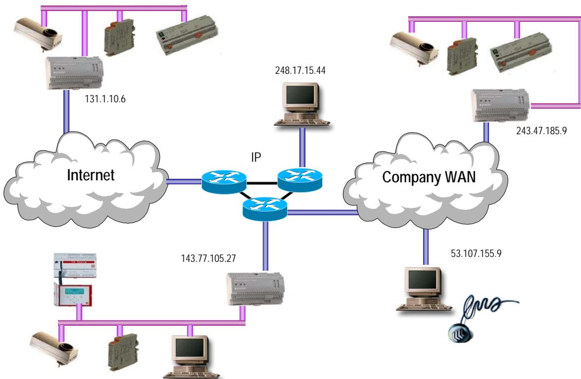
**LonWorks Packets are encapsulated within the TCP/IP packets.
