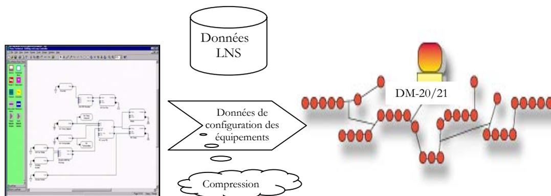
The above diagram illustrates the three steps necessary to successfully use the DM-21/21 to manage your network:
