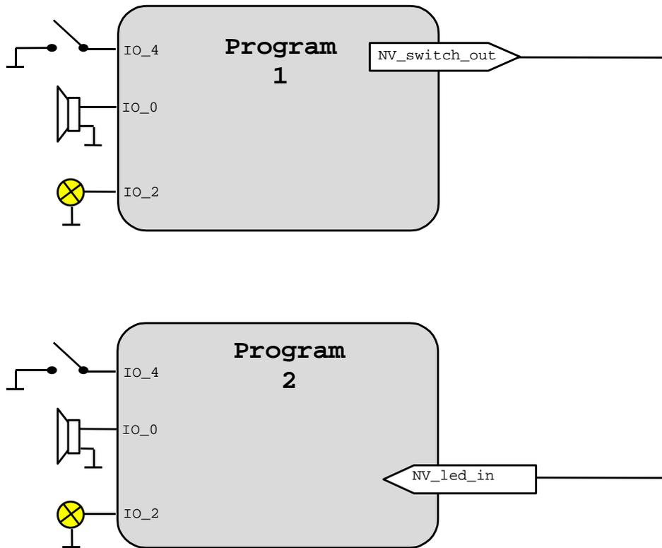
In order for both nodes to communicate, the network variables must be connected together using a network management tool /see section 22/. The network management tool is also needed to identify both nodes by sending network management messages to the nodes which would themselves reply by sending their Neuron ID<sup>6</sup>.
