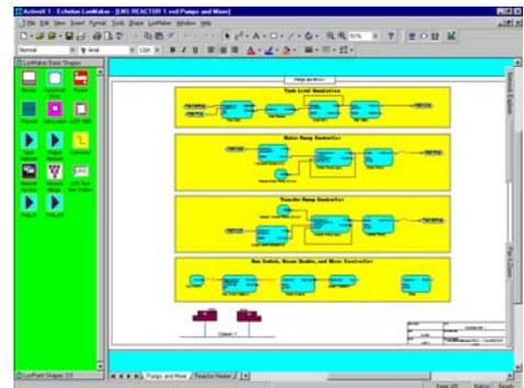
The LonMaker tool provides comprehensive support for LonMark® certified devices as well as other LONWORKS devices. The tool takes full advantage of LonMark features such as functional profiles, configuration properties, resource files, and network variable aliases.
