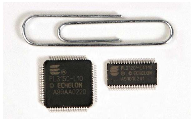
The powerline transceiver can automatically take care of the CENELEC access protocol which enables systems (sets of devices) from various vendors to share the same power cable and still communicate without interfering.
