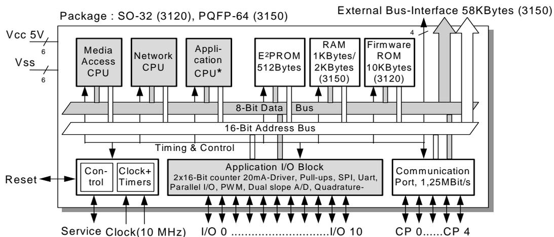
TOSHIBA offer various Neuron IC models in different package types and memory sizes: The model 3120 is a single chip Neuron – no external memory is required; the 3150 is an equivalent to a 3120 with the exception of its external memory interface used to store the firmware, program and application data.
