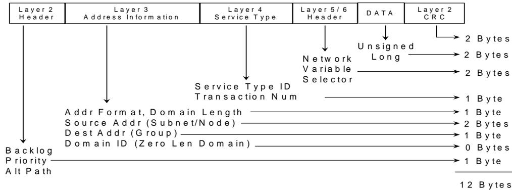
The data field may be up to 228 bytes long. The domain ID field may be 0, 1, 3 or 6 bytes long. In general, the protocol overhead is of constant length of 10 bytes.
