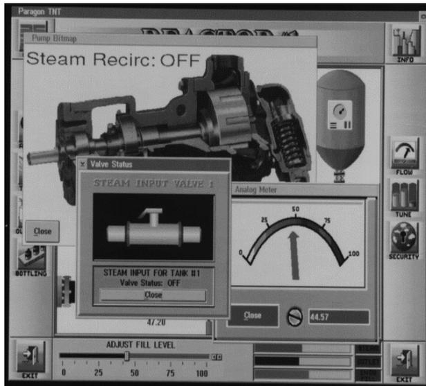
Screenshot of a LONWORKS network monitoring Software based on the LNS DDE server
