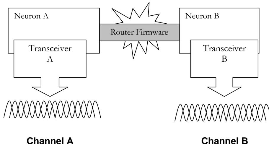
Routers are used to optimize packet traffic on channels. Packets generated on one channel are selectively forwarded to another channel if they contain address information referencing that channel.
