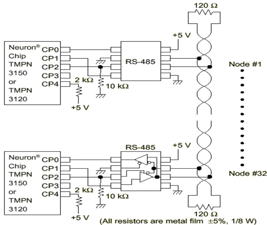
**\*All chips ground level must be within  $\pm 7$  V.**
